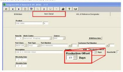
For complex assemblies, some components or sub assemblies may not be required until late in the production process. The "Production Offset" field allows you to specify how long this delay should be. This enables MRP to schedule this part the specified number of days AFTER normal production begins.
