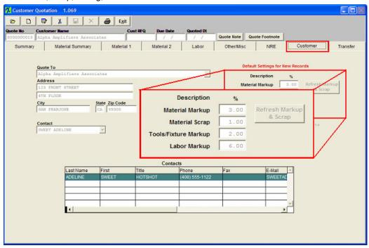
On the "Customer" tab users can set the default markup for a quote. They then have the ability to change the markup on each component. Additionally, if users would like to reset all markups on a quote they can use the "Refresh Markup & Scrap" button after making the necessary changes to the default values. This flexibility increases your competitive edge to help win the business.
